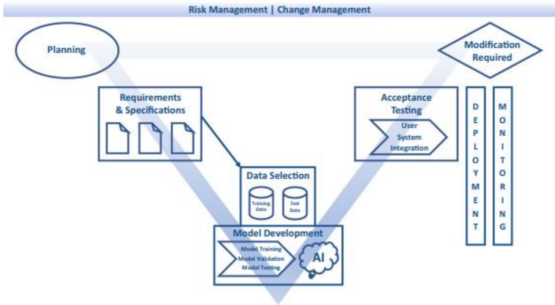
Fig. 3 Proposed ISPE GAMP® 5 methodology for validating artificial intelligence (AI)-based static systems in pharmacovigilance
